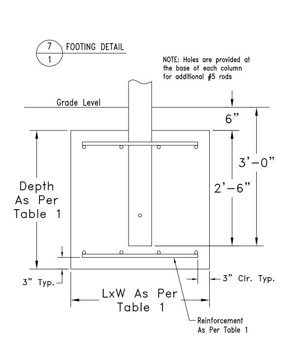
NOTE: A HOLE IS PROVIDED AT THE BASE OF EACH COLUMN FOR ONE #5 ROD.
